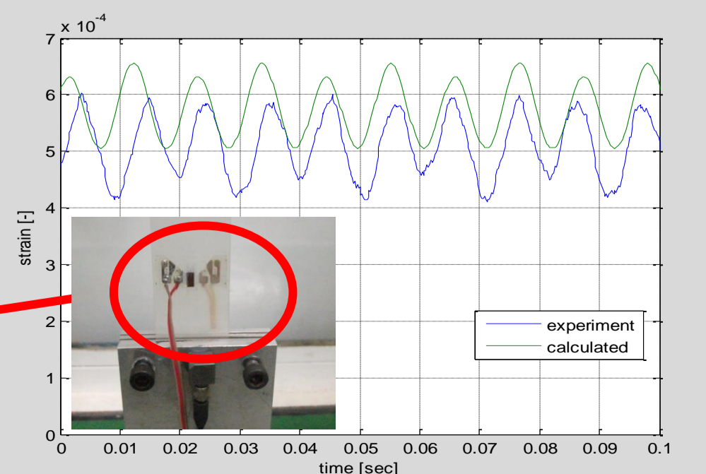
Time history comparison of strains, pretension=2.25 kg, airspeed=8.1 m/sec
